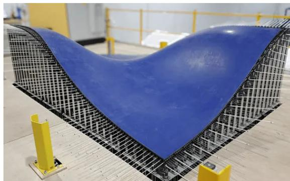
Figure 2. Example of an adaptive mould, from <https://www.bespline.ca/>
